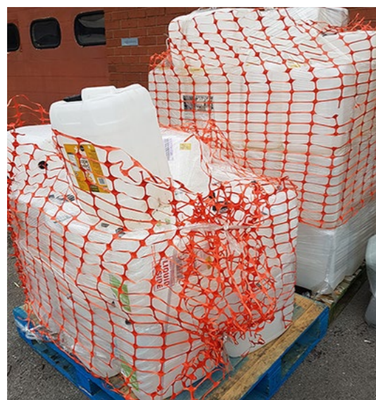
SESI Pallet Containment Prototype with Scaffold Net
